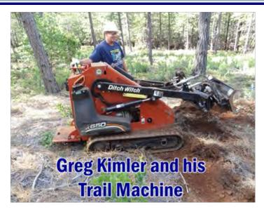
The Ditch Witch Model SK-650 trail machine is owned by Greg Kimler of Echo Valley Ranch. This highly efficient trail machine is only 36-inches wide, and is powered by a 20-hp diesel engine. The hydraulic blade is controlled by levers and knobs at the rear of the machine where the operator stands on a small platform. The trail machine is estimated to be 20:1 more efficient in machine-time versus manual chopping.
