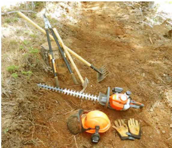
*At left:* Safety helmets and gloves were used with a variety of tools: a Husqvarna long-bar hedge trimmer to remove blackberry vines and brush; a Pulaski axe to chop out roots; a MacLeod hoe to remove pine needles and create rolling grade-dips; and long-reach loppers to cut roots and brush.
